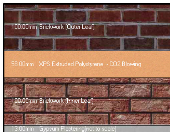
Figure 5 - An example of a standard South African outer wall (left) and one that complies with SANS 204 (right). In practice any materials can be used, as long as minimum insulation levels are achieved.
